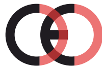
False CE Mark (too close)
