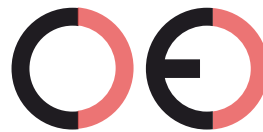
False CE Mark (too far)
